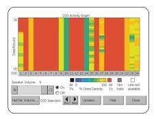
The DSO Activity Graph arranges the DSOs into columns. Time is the vertical axis and different densities are shown with different colors. With this unique feature, users can quickly verify the presence of traffic, signaling channels, etc., and how the data is changing over time.
