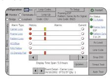
The YBT1E1 allows users to gather detail on any of the alarm or error events. Simply touch any of the red events and the instrument provides detail about the network event. This detail includes the number of events and the time of the event, and provides useful information to correlate network logs to field data.
